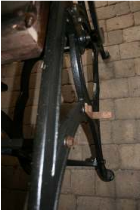
Note levitator stop is now a right angled piece of steel.
